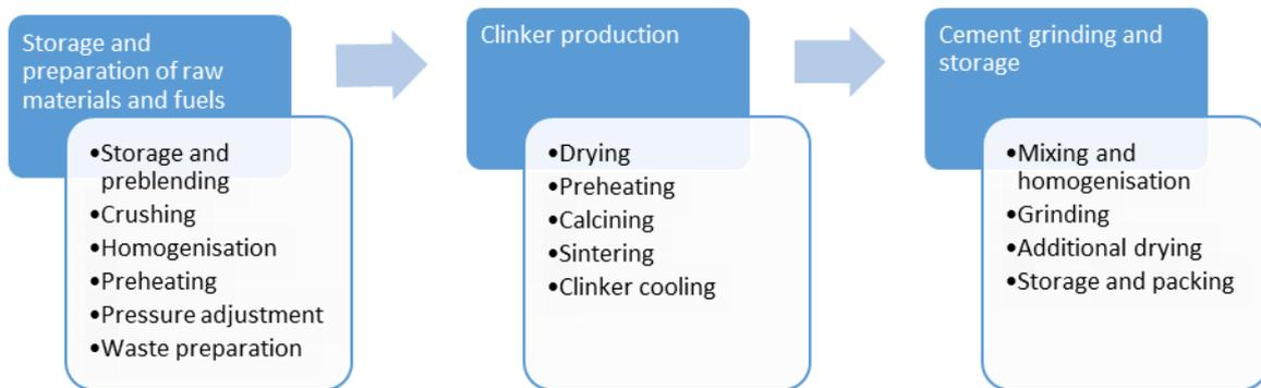
Figure 1: Cement production process.
