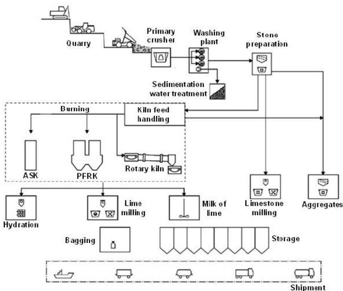
**Figure 4: Overview of lime manufacturing process.**
