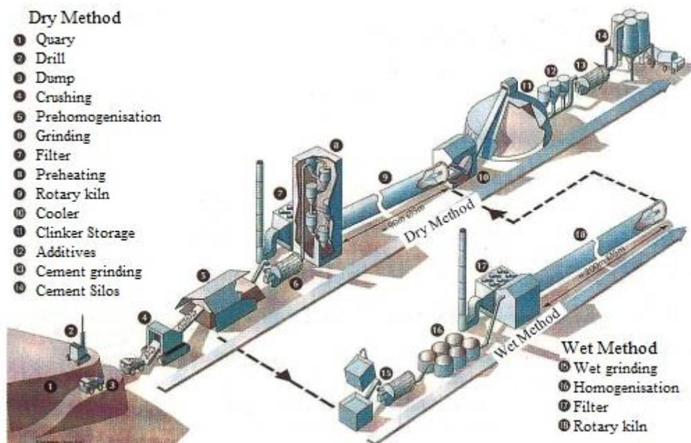
Figure 2: Scheme of cement manufacturing process.
