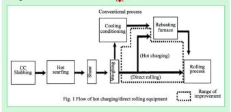
The image shows how the cooling step is skipped in the hot charging option.
